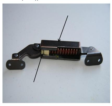
Excelsior Inc. provides a shim made out of HDPE that acts as a bearing surface against which the spring travels. This is applied to both commercial and home goods models. For commercial units Excelsior provides a rectangular shim made of Delrin® that the cam runs on. It acts as both a shim and a heatsink.
